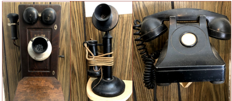
Left to right: Western Electric 250W crank wall telephone, 250W candlestick phone, and 302 model telephone with no dial.
